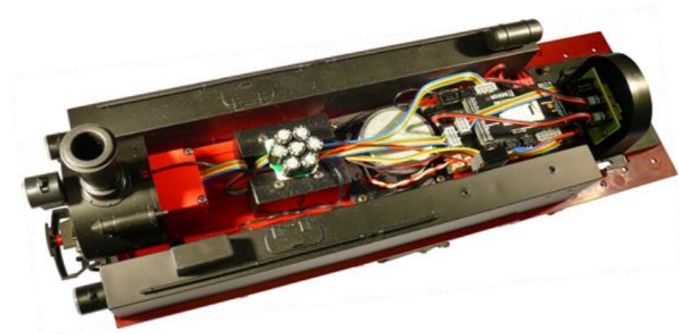
The upgraded locomotive: Goldcap-Module on the left, decoder on the right.
